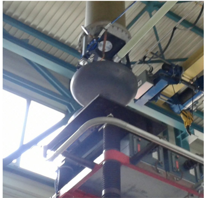
Spark gaps for laboratories with a high repeat accuracy (important for an accurate reproduction of test results)
